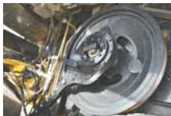
New reverser uses a ratcheting reversal system with a longer handle than the OEM wrench. It reduces the time and arm strength needed to reverse a plugged cylinder.
