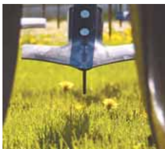
Finish Line Sweeps have a knife blade on the bottom that fractures the soil below, just as the point and wings fracture the soil above. The result is less soil compaction.
