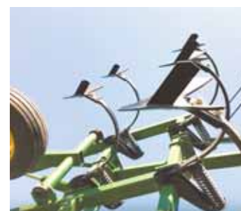
Finish Line Sweeps have a knife blade on the bottom that fractures the soil below, just as the point and wings fracture the soil above. The result is less soil compaction.
