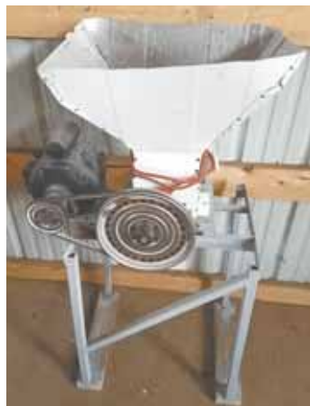
Corbin used armatures off junked car starters to make rollers for his small mill.
