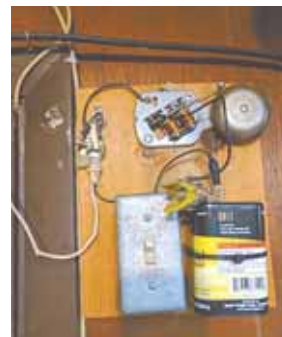
Burglar alarm was made from a 6-volt alarm bell, a pair of car ignition points, and a 6-volt lantern battery.
