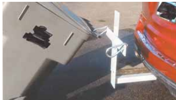
"Upright and cross arm" hitch lets Brinkhaus pull 2 garbage cans at a time behind his ATV or van.
