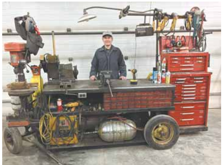
Glen Wasmuth's 10-ft. long "shop on wheels" has a 6-ft. tow bar with a caster wheel assembly at one end.
