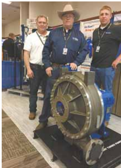
Ron Lounsbury says his Smart Turner Pump has no trouble handling manure from dairies that use sand bedding.
