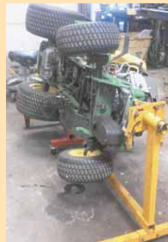
Lawn tractor rotisserie uses the pipe-in-pipe mounting heads off a pair of engine stands. "I can turn the tractor on its side or all the way over," says Podoll.
