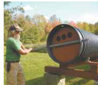
Four holes cut into lower end of culvert let Harwood turn it by hand.
