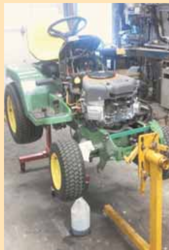
Lawn tractor rotisserie uses the pipe-in-pipe mounting heads off a pair of engine stands. "I can turn the tractor on its side or all the way over," says Podoll.
