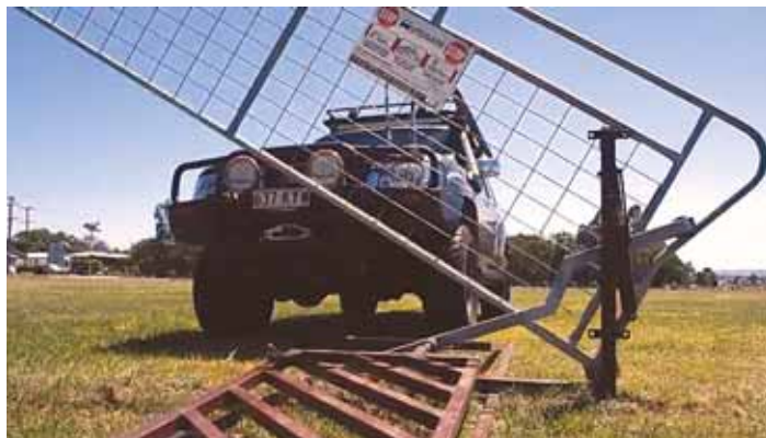
Automatic gate comes with a pair of steel ramps attached to a main frame assembly, and a hydraulic cylinder attached to hidden tension springs.
