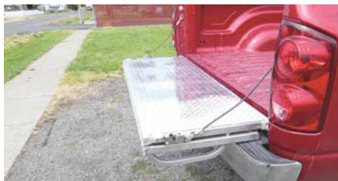
Fold-out loading ramp attaches to pickup just like the original tailgate. “It can't slip off, and it doesn't take up any room in the pickup bed,” says Colt Sherrer.
