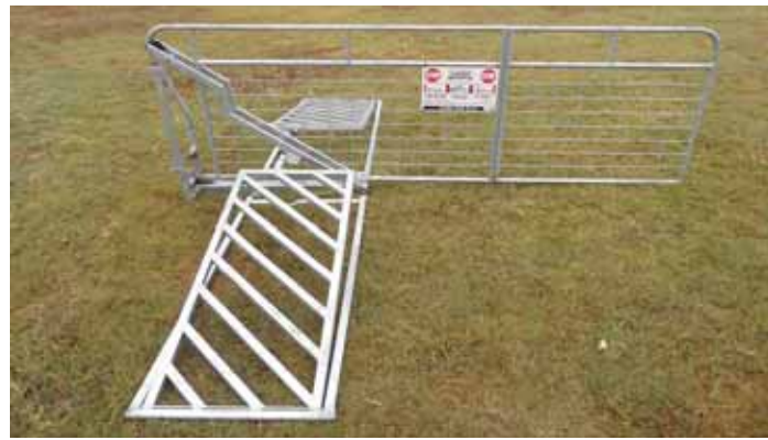
Down pressure on either ramp causes a hinged metal arm to act on the cylinder and force gate open vertically.
