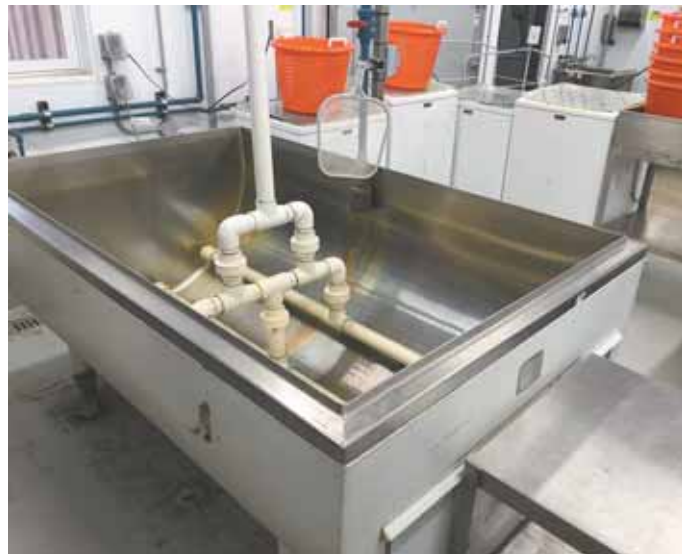
The Bubble produce washer is an old milk tank lined with perforated pvc pipes connected to a Jacuzzi pump.
