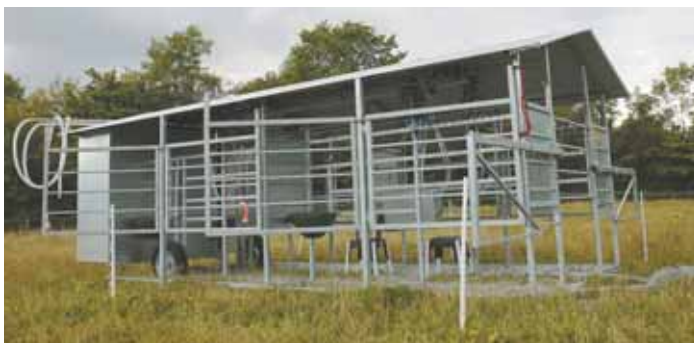
Mobile milking parlor consists of a milking trailer with stalls, milkers and a washing system as well as a support trailer with hot and cold water, a milk cooler, wastewater tank, and pto generator.
