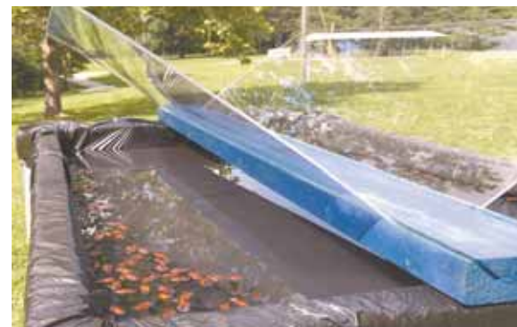
Black garbage bags wrap around a wooden basin, with 2 sheets of clear Plexiglas mounted at an angle above them.
