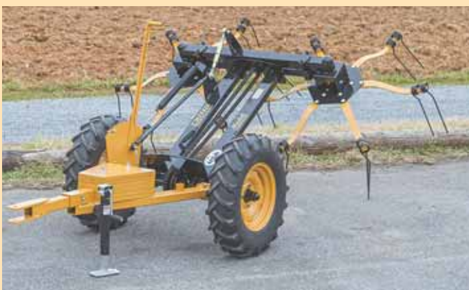
Each ground-driven tedder is designed for single teams of horses or can be used with a small tractor, ATV or UTV. Available with either steel or rubber-tired wheels.
