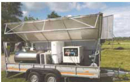
Mobile milking parlor consists of a milking trailer with stalls, milkers and a washing system as well as a support trailer with hot and cold water, a milk cooler, wastewater tank, and pto generator.
