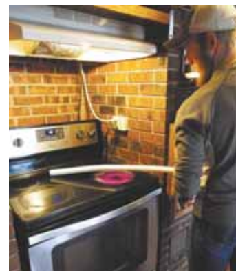
Caleb Howerton made a recurve bow for his wife out of a 5-ft. length of 1-in. dia. pvc pipe, using his stove top to heat and shape it.
