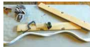
Once half of the pipe was heated, he used a 2 1/2-ft. long jig to flatten it at a taper. The process was then repeated on the other half of the pipe.
