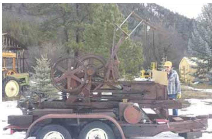
Bob Mayes made this giant can crusher out of an old IH stationary hay baler. A 3-ft. long metal pipe about 12 ft. up in the air comes down to crush the can.
