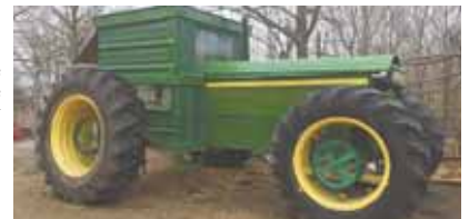
Chicken tractor's body is made from wood and metal. Eggs are gathered from nesting boxes by opening tractor side panels.
