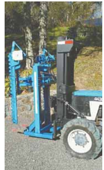
Gradek converted an old forklift to fit his New Holland tractor, and also converted his cane cutter into a freestanding unit with forklift tubes at the bottom.
