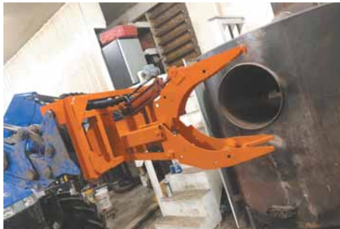
Jason Timm built log "clams" out of parts from an old 7-bottom White plow. The sides of the clam are 18 in. apart so wood can be sawed in firewood lengths while in the clam, and the remaining piece in the clam is also firewood length.
