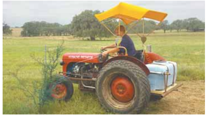
Bryan Albrecht converted the transmission on an old Ferguson TO-20 tractor to hydrostatic drive. A single foot pedal provides infinite forward and reverse control and is easy to use (above). He replaced the tractor's worn-out engine with a 22 hp. V-twin from Harbor Freight, and mounted a hydraulic motor on the transmission input shaft.
