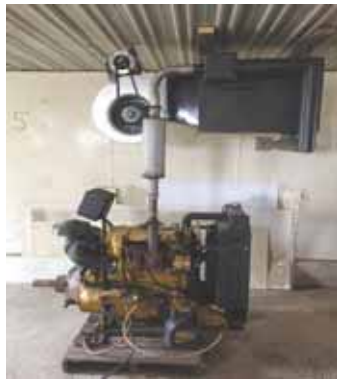
"Capture the Heat" unit uses engine exhaust to heat buildings. Exhaust enters box filled with baffles, then exits out the bottom and is piped outside.
