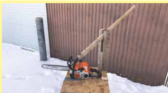
Wooden "pump handle" serves as a lever to pull chainsaw rope, which slips through a metal ring on end of handle.
