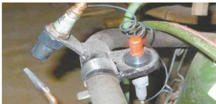
Piezo-electric ignitor is wired to spark plug on bracket that attaches to torch cart handle. "To light my cutting torch, I just hold it up to the spark plug and press the button," says Beardslee.
