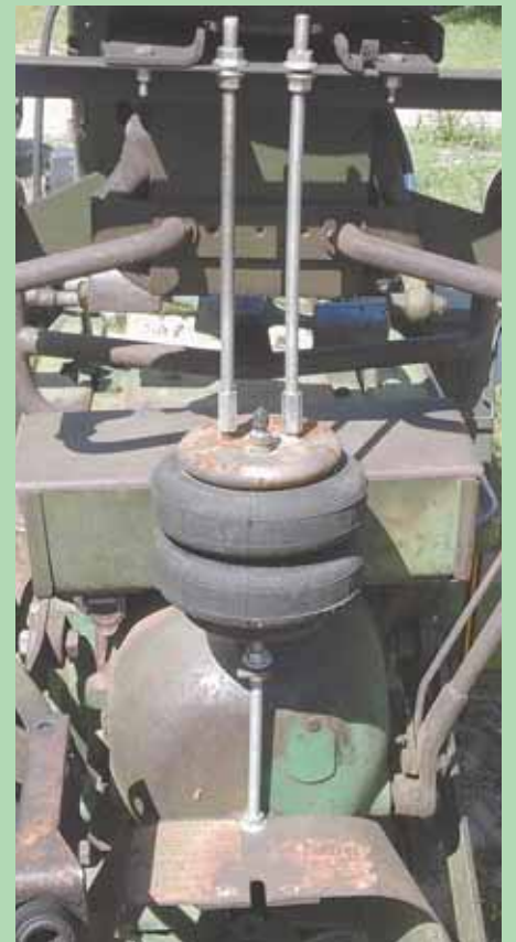
C. Roger Podoll made an air ride seat for his Oliver 770 using the airbag off a truck. It's mounted between tractor's pto shield and seat.
