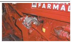
Ken Hall used the electric power steering motor from a car to add power steering to his Farmall "B". He cut 1 ft. out of tractor's steering shaft to attach motor.
