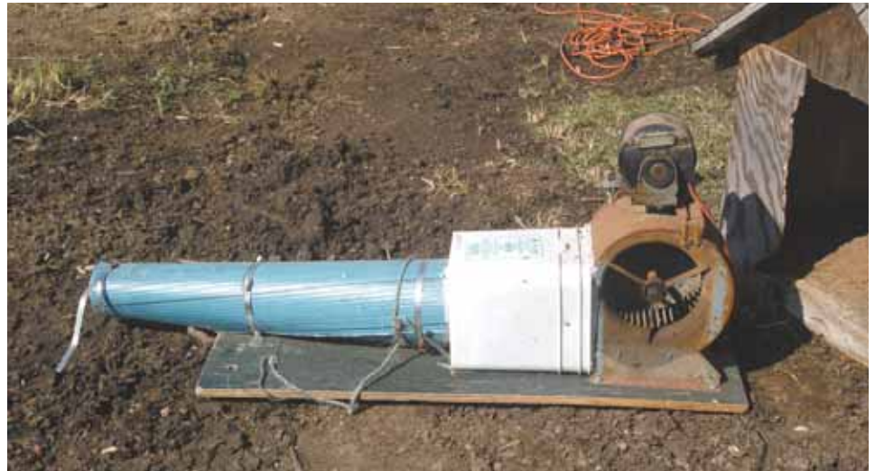
A squirrel-cage fan blows air through a makeshift funnel into the pvc pipe aerators. A timer turns fan on and off periodically.
