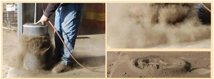
During tests on a pair of Deere 7750 tractors, one tractor's air filter was cleaned once a day. Nearly 5 lbs. of dirt was removed daily and the tractor used 58 gal. less fuel per day than the tractor with the dirty filter.
