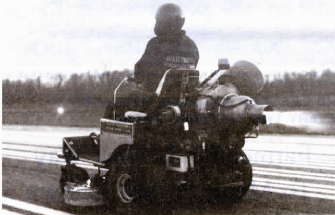
Evans mounted 150 hp jet turbine out of Chinook helicopter on back of stock mower.
