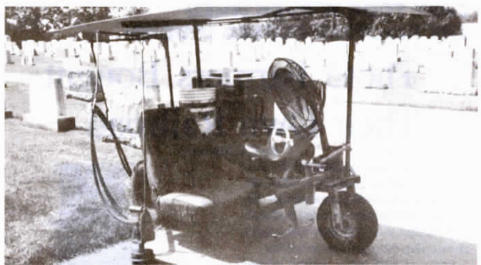
The 3-wheel trimmer is powered by a 10 hp Wisconsin engine. Note fan in front.
