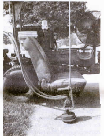
Trimmer is fitted with free-swinging "weed eater" cutterhead that Zimmerman guides with his right hand.
