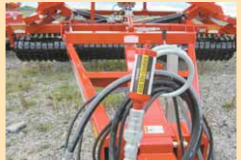
When inactive hoses are coupled to the Hose End Chamber, it relieves hydraulic pressure buildup in the hoses.
