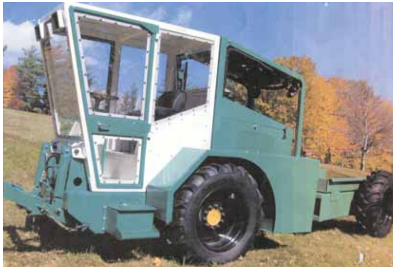
Maury Collins's PRO III 4-WD articulated tractor is powered by a 90 hp. Deere diesel engine. Tractor's rear half is available for use as a flatbed, dump box or log bed.
