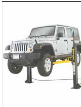
Portable 2-post lift hooks up to a mobile power unit and can lift 6,000 lbs. up to 4 ft. high in 30 secs. For something smaller you can use just one lift post with an optional lift attachment.
