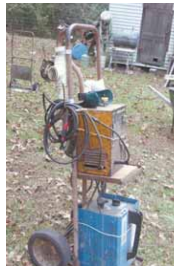
Modified hand truck holds 2 welders as well as welder cables and welding rods.
