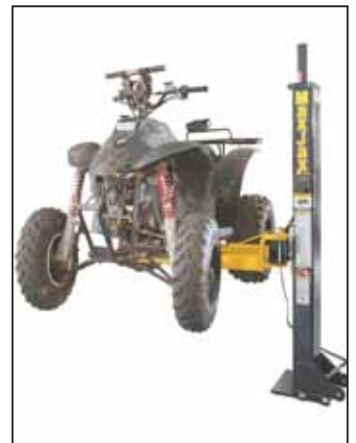
Portable 2-post lift hooks up to a mobile power unit and can lift 6,000 lbs. up to 4 ft. high in 30 secs. For something smaller you can use just one lift post with an optional lift attachment.
