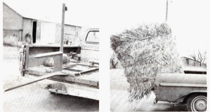
Bale spear is operated from pickup cab; tailgate must be removed.
