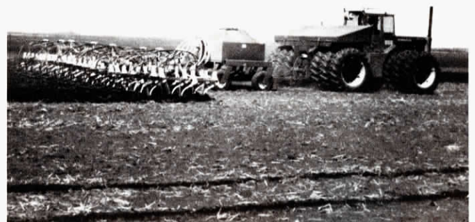
Seed-Air doesn't interfere with foldup of wings for transport; liquid fertilizer can be adapted to system.
