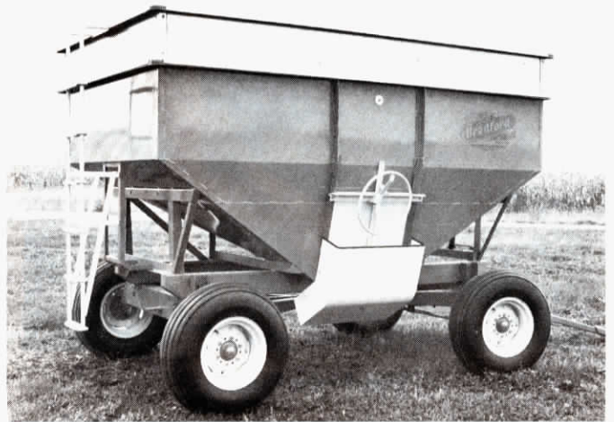
Converted wagons can be changed back to side-unload by removing two bolts to remove the chute.
