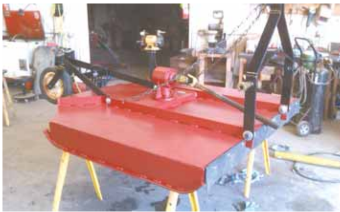
Dale McLaen rebuilt an old 3-pt. mounted mower by stripping it down and building a new deck out of 1/4-in. steel.
