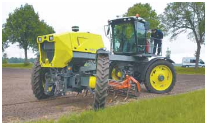
Track width can be adjusted between 7 - 10 ft. on-the-go, and there are 5 positions for attaching tools and implements.
