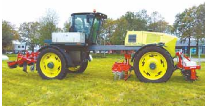
The MultiToolTrac, electric/diesel, hybrid tractor has a completely electric power train that makes use of 4 electric wheel motors.
