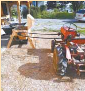
Keim's small home-built thresher is belt-driven off his subcompact tractor. Bundles of grain are put in the box and the top closed, then a shaft with chains flails the grain.
