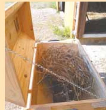
Keim's small home-built thresher is belt-driven off his subcompact tractor. Bundles of grain are put in the box and the top closed, then a shaft with chains flails the grain.
