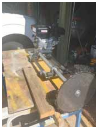
Loader-mounted brush cutter uses a Harbor Freight engine, which shaft-drives a 12-in. dia. Beaver Blade attachment off a DR walk-behind trimmer.
