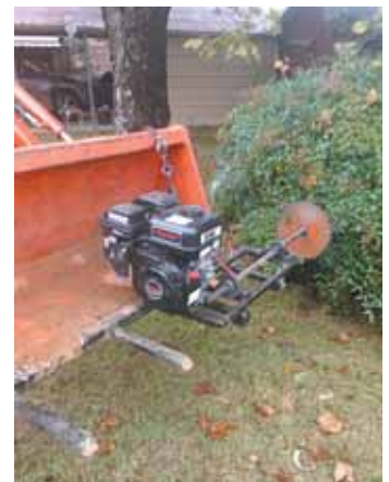
Loader-mounted brush cutter uses a Harbor Freight engine, which shaft-drives a 12-in. dia. Beaver Blade attachment off a DR walk-behind trimmer.
