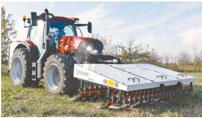
XPow machine produces pulsating electricity with a rear-mounted generator driven by the tractor pto. It kills weeds almost immediately.
