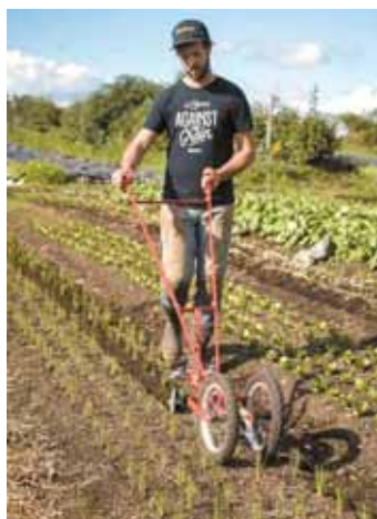
Twin wheels on hoe straddle the row, making cultivation easy. Wheels also quickly attach to a variety of other tillage tools.
