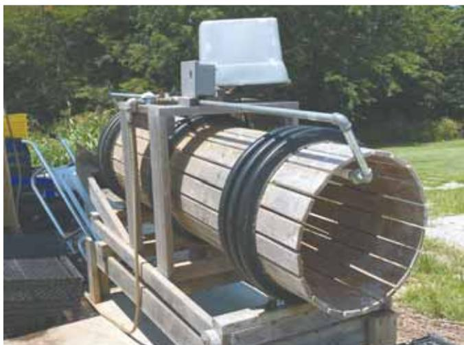
Pieces of corrugated drainage pipe provide tracks for roller.
