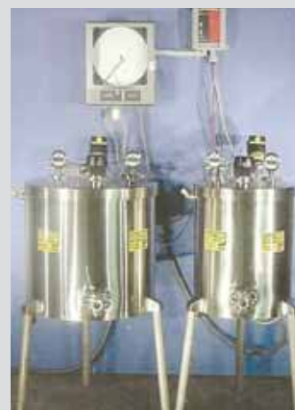
Vat pasteurizer can pasteurize milk and also make cheese.
