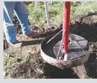
McLaen used his home-built post hole clean-out bit this fall to pull gooey, loose clay out of 24-in. dia., 40-in. deep augered holes. It worked like a charm.
