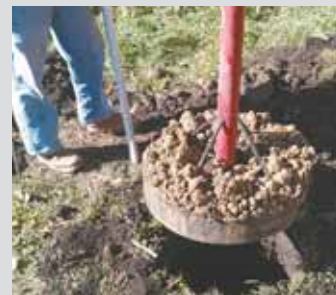
McLaen used his home-built post hole clean-out bit this fall to pull gooey, loose clay out of 24-in. dia., 40-in. deep augered holes. It worked like a charm.
