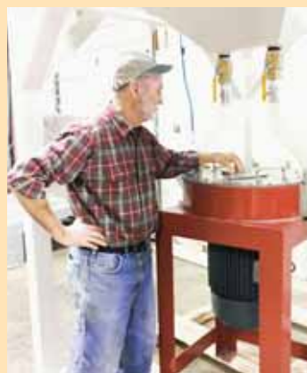
Mill uses high-velocity airflow and a high-speed spinning drum to force grain against tiny teeth on the inside of the drum, busting kernals apart.
