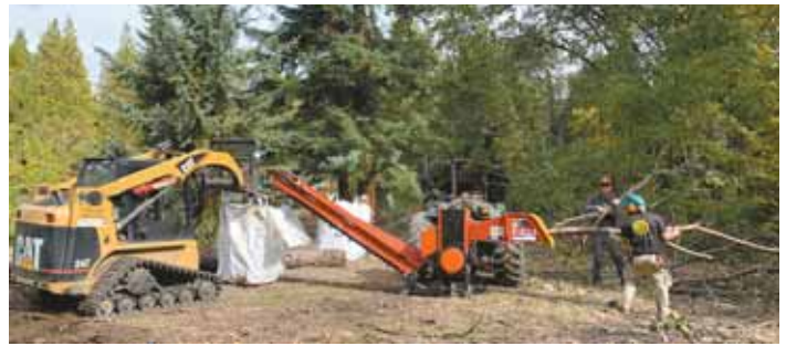
The 3-pt. mounted Wood Chunker chops 2 to 6-in. dia. branches and small trunks into 6-in. long chunks of wood. It can be equipped with an optional conveyor.
