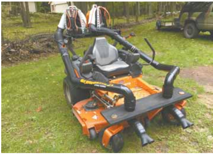
A pair of Stihl backpack leaf blowers mounted on back of mower move air forward through lengths of 4-in. pvc pipe.
