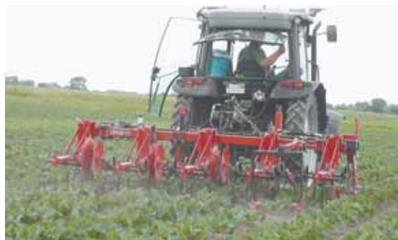
Steketee Finger Weeder comes with a wide variety of finger types and sizes that all slip onto the same hub.
