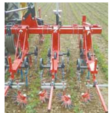
Fingers mount on 9-in. long shanks that are fixed to a steel disc, dislodging weeds as they travel down the row.
