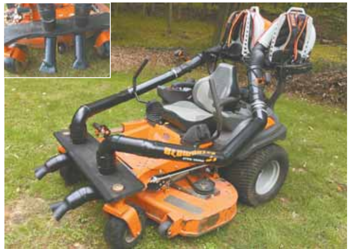
At front of deck, 90-degree fittings direct the air through blower nozzles that hook up to the pipes. Since these photos were taken, O'Neil replaced the split nozzles with a fan-type tip (inset photo above).
