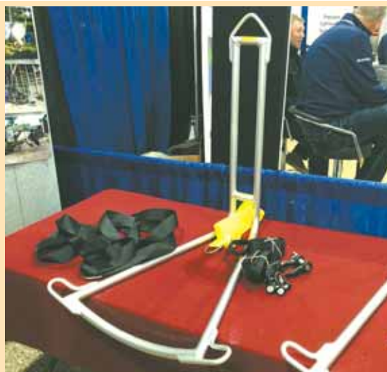
Chair-like frame, combined with a strap harness, supports cow. It can be used with a loader bucket or forks.
