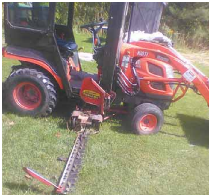
Belly-mount sicklebar mower mounts alongside Peloquin's 24 hp. loader tractor, and is belt-driven off tractor's front pto.
