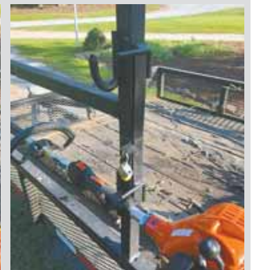
Rack is welded onto one side of trailer. Operator lays tool across a pair of steel hooks, then folds a hinged bar against upright and locks it in place.
