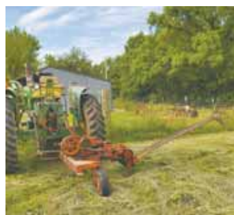
McCarty restored this old Allis Chalmers 2-pt. mounted sicklebar mower and uses it to cut 2 acres of hay. He likes the gearbox drive.
