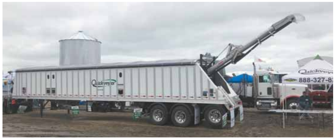
Semi-truck mounted auger makes it easy to load large fertilizer applicators or seed boxes. A 4-direction, swinging discharge chute on back can be controlled with a remote or with push buttons on side of trailer.
