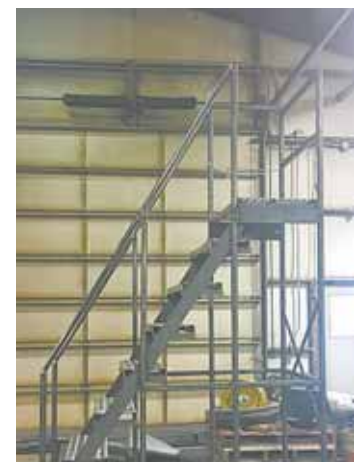
Driver places skid loader forks under horizontal cross bars on stairway to move it around.
