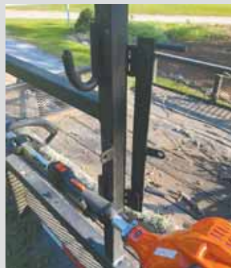
Rack is welded onto one side of trailer. Operator lays tool across a pair of steel hooks, then folds a hinged bar against upright and locks it in place.
