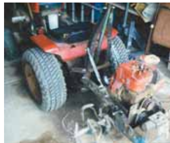
Walk-behind rototiller’s drive system mounts on an angle iron frame that attaches to a “4-pt.” hitch equipped with a single hydraulic cylinder.
