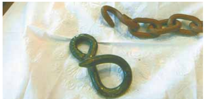
Homemade pigtail hooks onto a chain wrapped around gate and post to keep gate shut. “It’s easy to put on and take off, and it won’t jump out of the chain,” says Seltzer.
