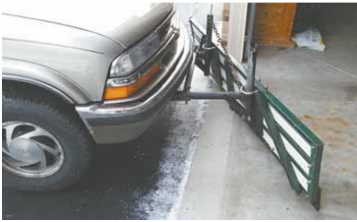
Dual angle attachment system is supported by a pair of horizontal pipes unequal in length. Scheibengraber can switch blade angle to the left or right by pulling 2 pins from receiver tubes mounted on front of vehicle, then swapping the pipes.
