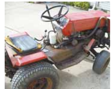
Billings uses a valve on tractor’s operator platform to raise and lower rototiller. A hydraulic pump and valve mount on side of tractor.
