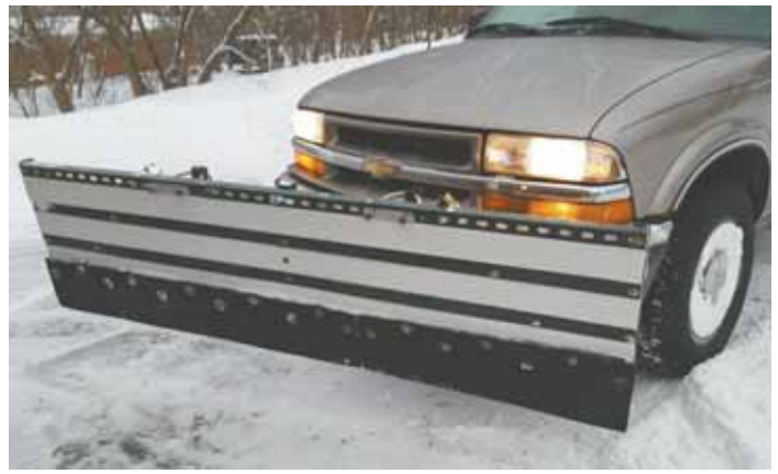
He used 2 by 4's and steel Unistrut sections to make the blade and added a rubber scraper at bottom. Blade hinges up and down on U-bolts, allowing it to slide on driveway when backing up.
