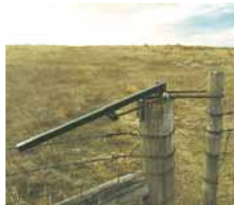
Lever automatically pulls gate end post tight against anchor post.
