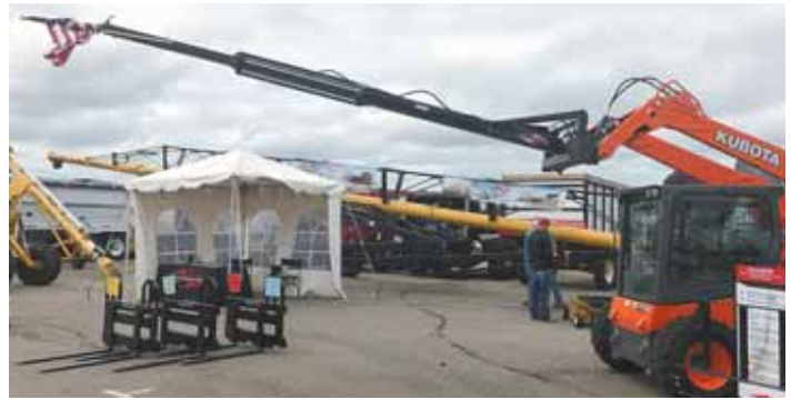
Skid loader-mounted Tele-Boom extends from 8 1/2 to 30 ft. Multiple add-on tools are available.
