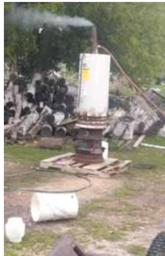
Wood-burning chicken scalding was made from an old water heater and a truck tire rim stove. Water runs into heater through a garden hose.
