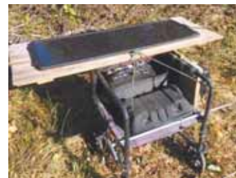
Wheelchair makes it easy to move solar-powered fencing system from field to field. It serves as a stand for the solar panel, car battery, and a photovoltaic controller that mounts on side of wheelchair.
