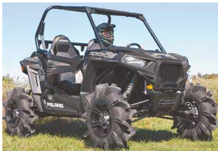
Assassinator Mud Tires come with 3-in. deep lugs that provide extreme grip in thick mud. The company says the tires ride smooth enough to be great for trail riding.
