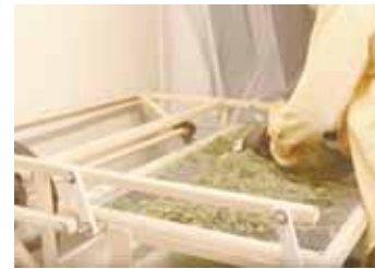
Herbal tea business uses hoop houses made from recycled silo rings covered in plastic (top left). A home-built motorized shaker table separates leaves and flowers from stems (top right). Home-built solar-powered dryer (below left) removes moisture. Screened material is stored in DiMaggio's farm house basement.
