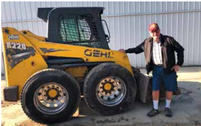
Al Hernke mounted larger wheels fitted with truck tires on his skid loader, providing it with extra clearance and more speed.
