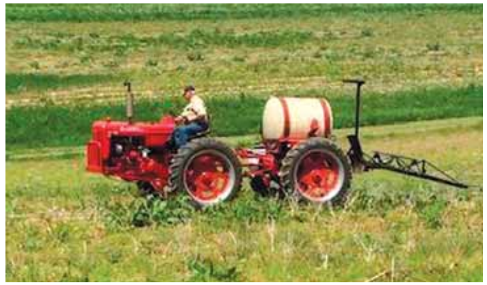
Tractor is powered by a 40 hp. diesel engine out of a junked Ford 3000 tractor. "Works great to spray corn and potato crops," says Davis.
