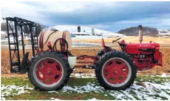
To join the rear ends, Davis built a hinged frame. He then ran a driveshaft from the original pto on the front rear end to the back rear end.
