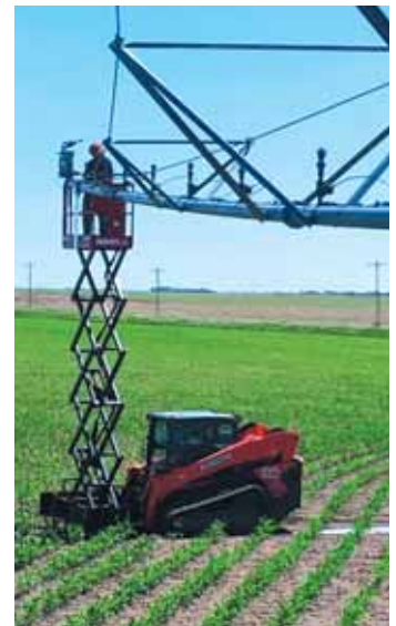
Scissor-lift attaches to tractors or skid loaders, providing a safe platform for working on grain bins or center pivot booms and many other jobs.
