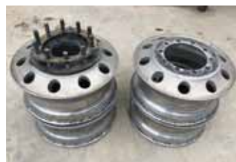
He made adaptor rings from scrap metal to mount the larger wheels to the hubs.
