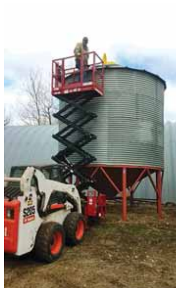
Scissor-lift attaches to tractors or skid loaders, providing a safe platform for working on grain bins or center pivot booms and many other jobs.
