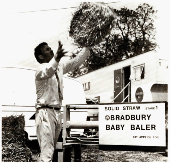
An English firm (Joseph Bradbury and Sons, Springwood Industrial Estate, Rayne Road, Braintree, Essex, Eng.) is experimenting with a Baby Baler. It compresses conventional bales to one-third their original size at rate of 7 per min.
