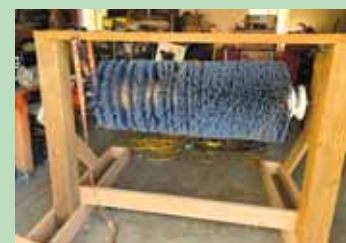
Hydraulic-driven street sweeper brush strips flower buds and leaf material off fresh cut hemp.
