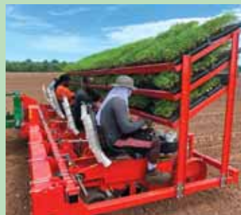
C&M transplanter comes with big cups and trays that can handle hemp seedlings up to 24 in. tall.
