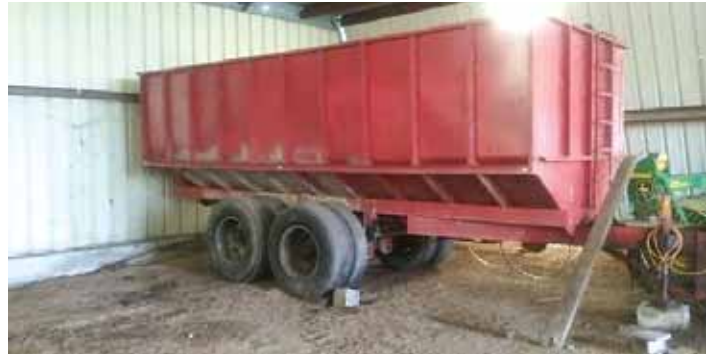
William Davis used the running gear from an old tandem axle semi trailer to build this 500-bu. rear-unloading grain hauler.
