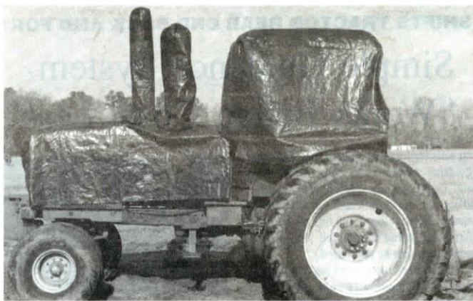
Separate pieces of waterproof nylon material cover cab, hood, and exhaust pipe.
