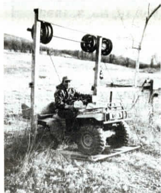
Pierson used three old car wheel rims to build gate that automatically opens and closes from either direction.
