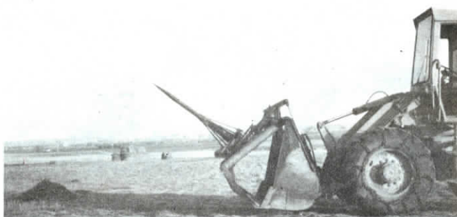
Rotating bale spike mounts on back side of grapple fork, allowing fork to be used normally without removing spike.
