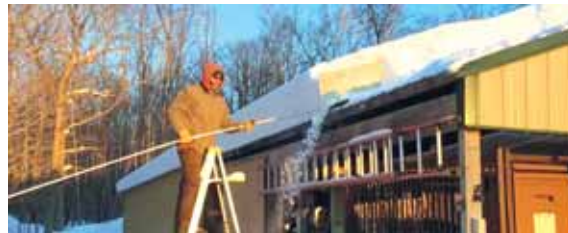
Snow removal tool consists of 2 pieces of metal siding attached at right angles to the end of a long pole.
