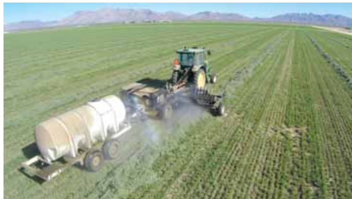
Machine injects pressurized hot water and a softening agent to the underside of hay windrows, reducing leaf shatter and loss.
