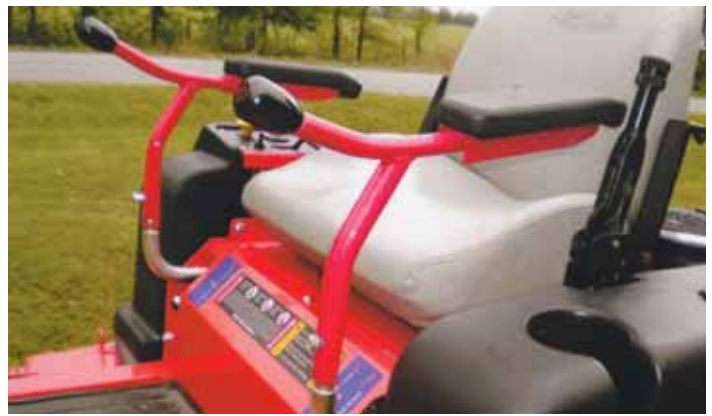
The operator can also control the machine by pushing a pulley on the arm rests alongside the seat.
