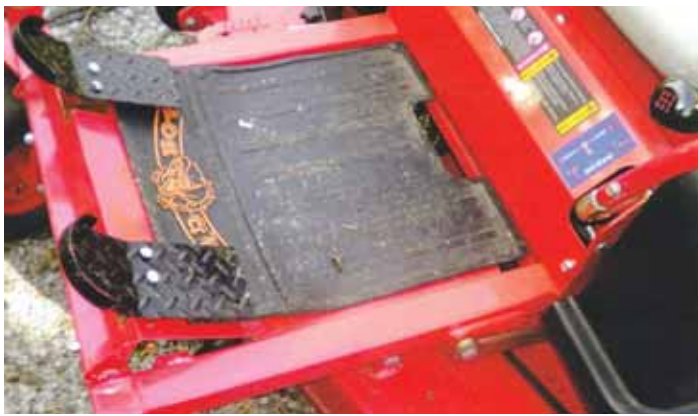
Pushing on toe portion of foot pedal controls forward movement, and pushing down on heel portion controls reverse. Pushing down farther either way controls speed.
