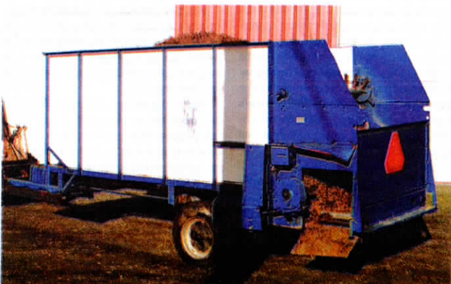
The 10-ft. long, 5-ft. wide wagon is equipped with a two-way cross conveyor on back. Lohman uses a skid steer loader to push wagon down alley, unloading silage out one side onto floor. Once he reaches end of alley he flips a toggle switch to reverse conveyor direction, then unloads feed out other side as he pulls wagon back out of barn.
