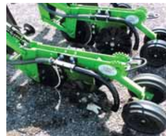
Biomass Builder knives in fertilizer while cover crop tubes drop seed behind wavy coulters.
