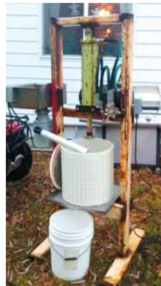
Electric-operated garbage disposal crushes apples into pulp. A hydraulic-powered press then squeezes out the juice through hundreds of holes drilled into a big diameter plastic pipe.
