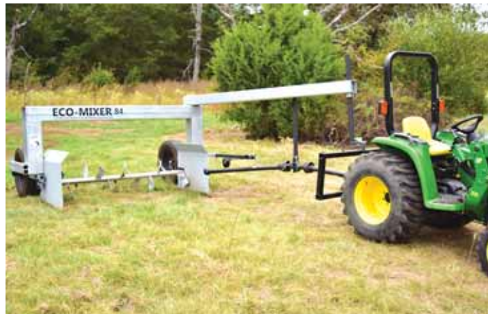
Compost turner is equipped with a tubular agitator shaft fitted with 9-in. paddles, and can handle a windrow about 3 ft. high by 6 ft. wide.
