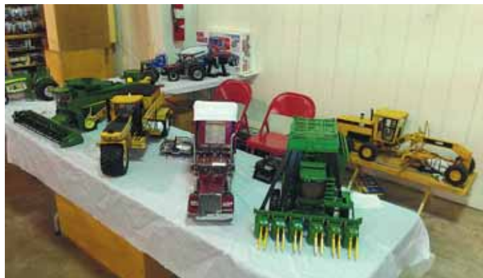
Denson's 1/16-scale, remote-controlled farm toys are equipped with electric motors, miniature gears, hydraulics, and radio receivers to work like real equipment.
