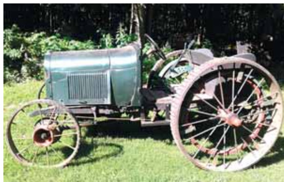
John Crofoot bought this 1928 Ford Model A tractor, which had been put together using a Sears kit that converted the Model A car to a tractor.
