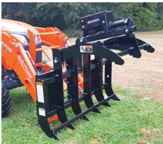
Electric grapple for subcompact tractors is operated by a 12-volt linear actuator.
