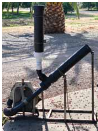
Modified backpack leaf blower blasts predator mites into walnut trees to attack other problem mites.
