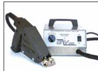
Nextire grooving gun heats a horseshoe-shaped razor blade that creates grooves in tires up to 1 in. wide and 1 in. deep.
