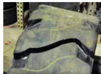
Nextire grooving gun heats a horseshoe-shaped razor blade that creates grooves in tires up to 1 in. wide and 1 in. deep.
